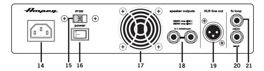
18. SPEAKER OUTPUTS: These 1/4" TS Speaker Output jacks supply speaker-level power to the speaker cabinet. The rated power output is 250 Watts RMS into 8  $\Omega$ , or 350 Watts RMS into 4  $\Omega$ .
